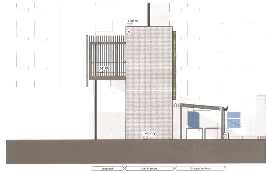
2. Side Elevation Towards MSCP - Bridge Link & Stair/Lift Core
